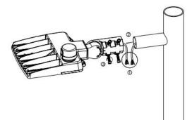
Step 2 Tighten the screws on the sides of the arm and then power on.
