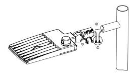
Step 2 Tighten the screws on the sides of the arm and then power on.
