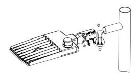
Step 2 Tighten the screws on the sides of the arm and then power on.
